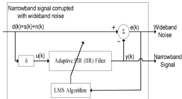
Fig. 3, Block diagram of Adaptive noise cancellation technique [10].
