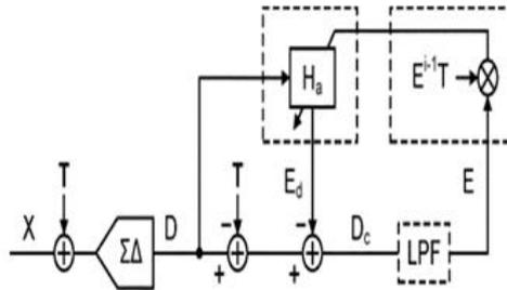
Fig. 4, Block diagram of harmonic distortion canceller [9].
