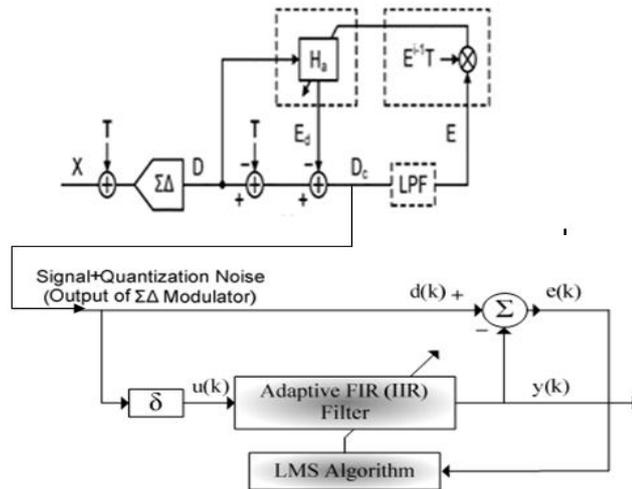
Fig. 5. Block diagram of proposed technique
