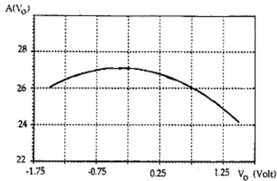
Fig. 1. Amplifier dc-gain characteristic as a function of the output voltage [11].
