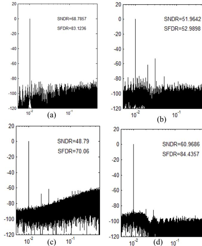
Fig. 6. Simulation results of a 5-bit first-order modulator After calibration : ( a) ANC with  $A_{\max} = 1e8$ , (b) ANC with  $A_{\max} = 20$ , (c) harmonic canceller, (d) combination of both technique.
