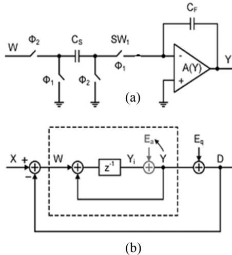
Fig. 2, (a) switched-capacitor realization of the integrator, and (b) the model with considering distortion signal [9].
