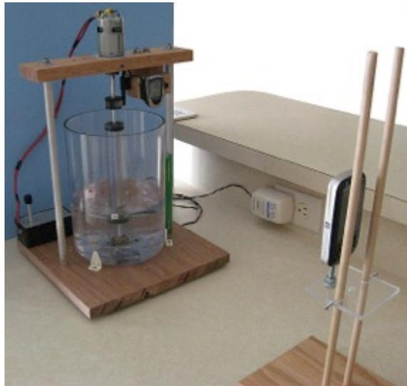
FIG 1. Experiment with central cylinder rotating at 15 Hz.
