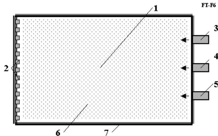
**Fig.3.** Conceptual diagram for installation producing AB-Matter. Notations: 1 – installation; 2 –AB-Matter (an extremely thin thread round bar, tube, net) and form mask; 3 – neutron source; 4 – source of charged particles (protons, charged nuclei), accelerator of charged particle, throttle control, beam control; 5 - source of electrons, accelerator of electrons, throttle control, beam control; 6 – cloud of particles; 7 – walls reflect the neutrons and utilize the nuclear energy.
