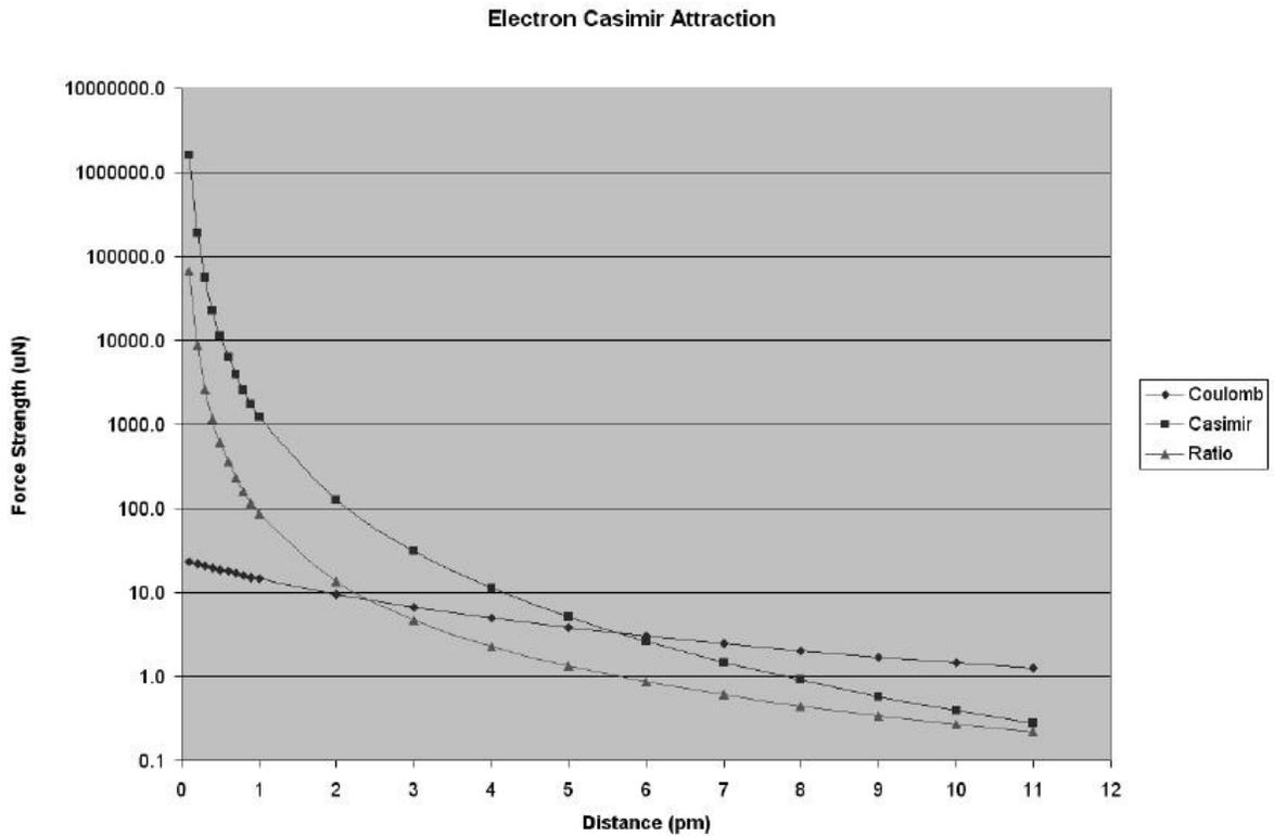
**Figure 1** Chart comparing the Casimir attraction versus the Coulomb repulsion between two electrons. The data was plotted with a logarithmic Y scale given the rapid change in the Casimir force for distances less than 2pm. The ratio line crosses 1.0 between 5pm and 6pm indicating net attraction at closer distances.
