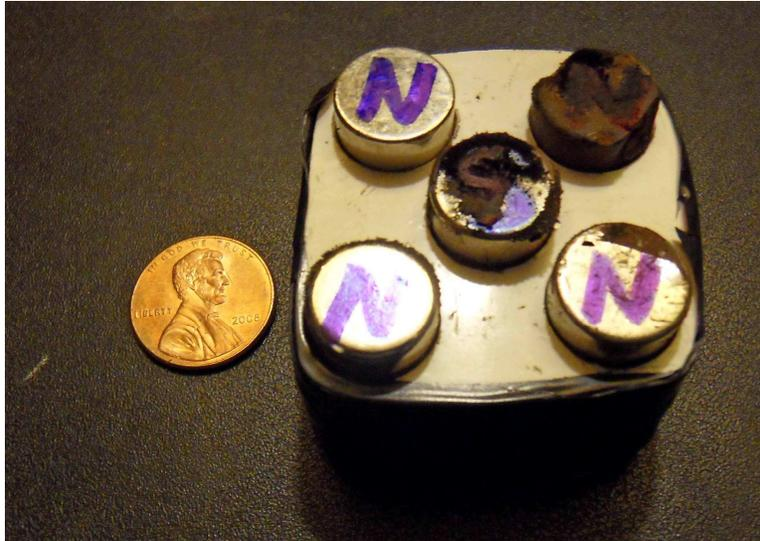
**Figure 4 - Alignment of five neodymium magnets.**
