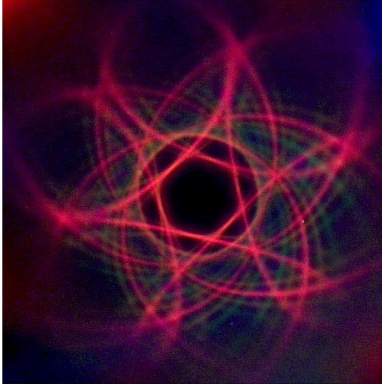
**Figure 11 - Single magnet LED operation, note the even pairs of bright lines.**
