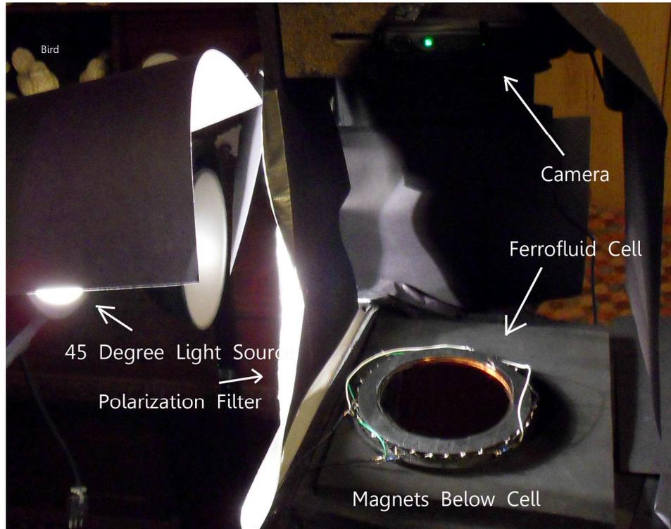
**Figure 2 - Experimental setup with 45 degree light source.**
