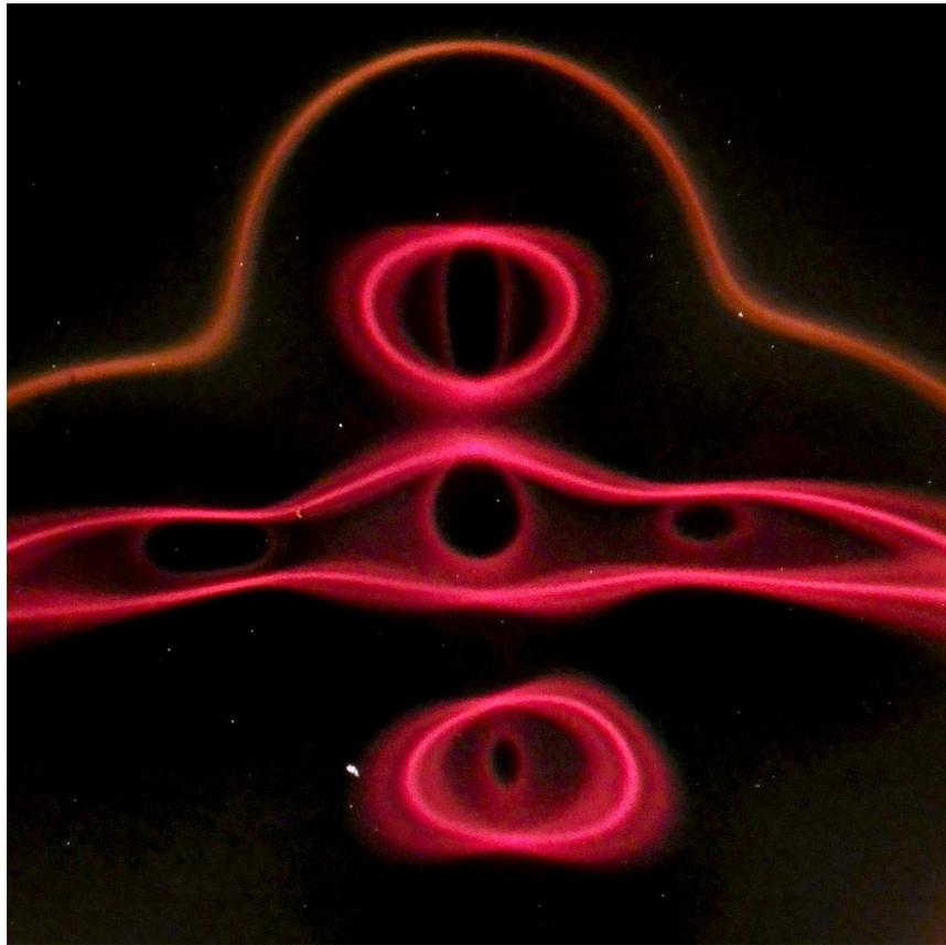
**Figure 8 - Same magnets as the other figures, all aligned north poles.**
