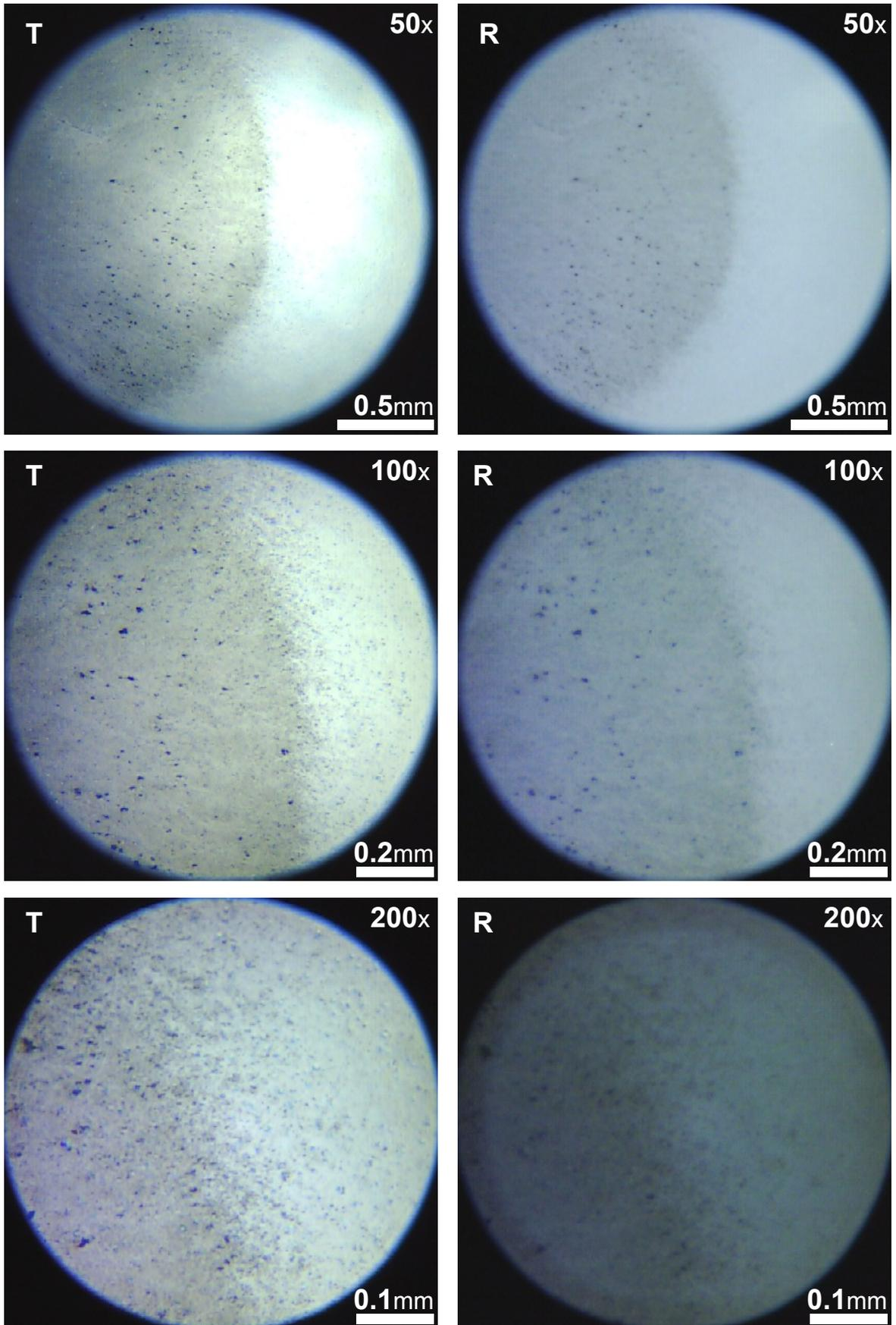
**Figure 6.** Microscopic images of polyester film (labeled as “26”) near the edge of the deposit. “R” stands for Reflection mode; “T” stands for Transmission mode.
