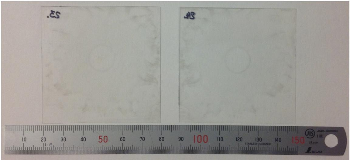
**Figure 3.** Polyester films (labeled as “23” and “24”) after the control experiment (i.e. after the contact with pristine ink; no table salt in the ink).
