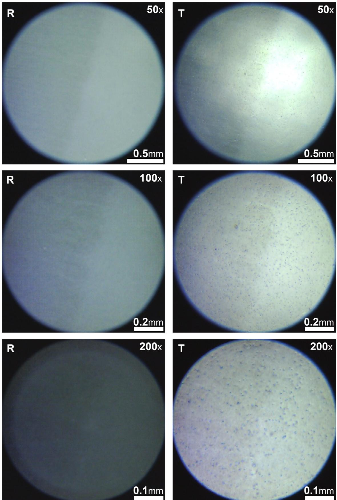
**Figure 5.** Microscopic images of polyester film (labeled as “25”) near the edge of the deposit. “R” stands for Reflection mode; “T” stands for Transmission mode.
