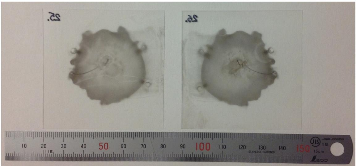
**Figure 4.** Polyester films (labeled as “25” and “26”) after the experiment (i.e. after the contact with ink, which contains table salt).
