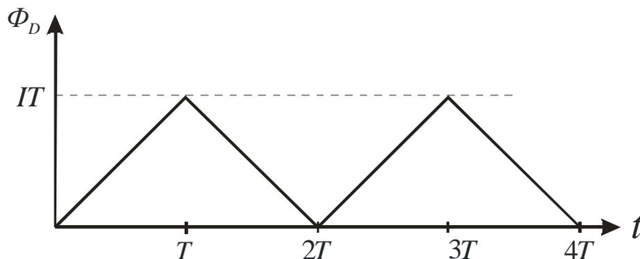
Fig. 4. Dependence of the electric flux on the time for the shortened transmission line.
