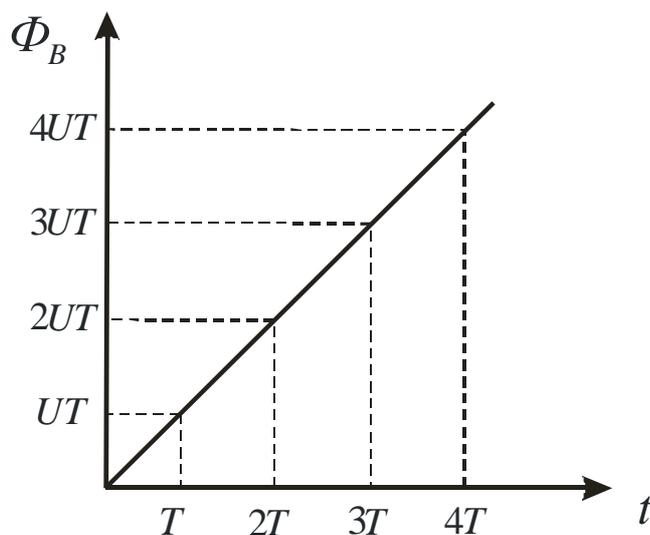
Fig. 3. Dependence of magnetic flux on the time for the shortened transmission line.
