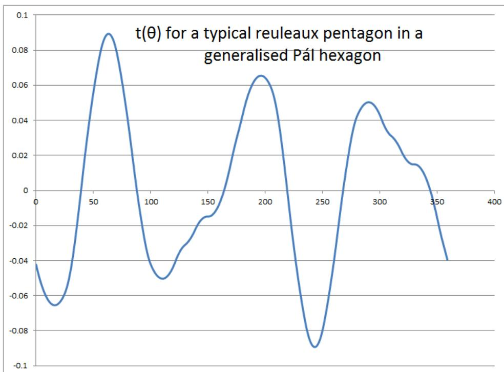
Figure 7 offset function for a typical Reuleaux pentagon
