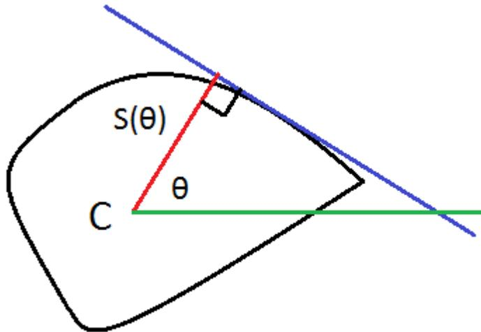
Figure 6: support function for a closed curve
