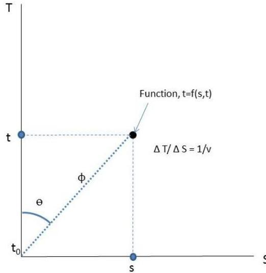
Figure 7 There should be no difference in representing space as the horizontal axis and time as the vertical axis, but since velocity is defined as  $v \stackrel{\text{def}}{=} \Delta S / \Delta T$  the line representing the change in one with respect to the other is the inverse of velocity.
