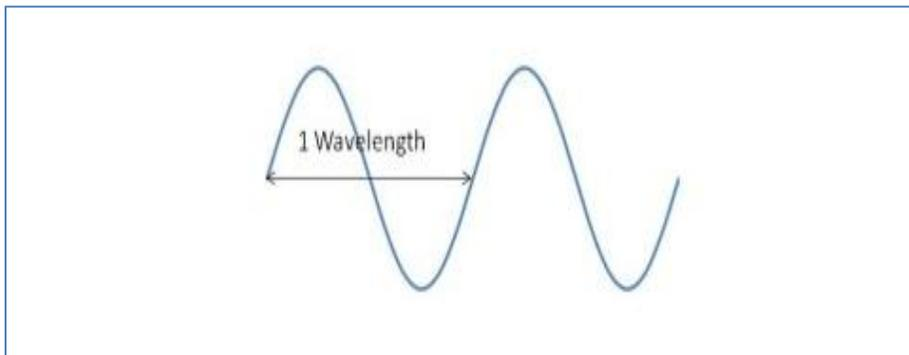
Figure 2 A wave can serve as a standard measure of space by defining one unit of measure as the distance between the beginning and end of one cycle.
