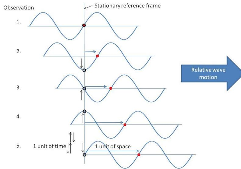
Figure 3 A stationary reference point allows motion of the same wave as to be used as a time standard. Each wave in the figure represents a snapshot as the wave moves to the right (red dot) and the intersection of the wave with the vertical line (small circle) moves down to the minimum, up to the maximum and back to the starting point. One unit of time is then defined as the duration between the beginning to the end of the cycle.
