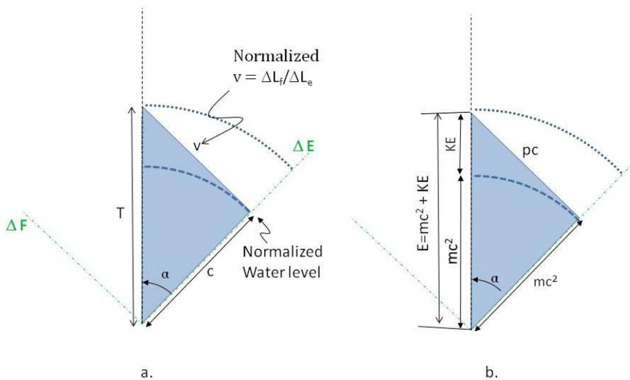
Figure 16 (a) The graphical representation of the water glass analogy, which level increasing at a constant rate equal to the conversion factor,  $c$ . (b) This diagram is the text-book example taken from Halliday and Resnick Fundamentals of Physics 4th ed, ch 42 as a mnemonic device for remembering the relativistic relations between rest energy, kinetic energy and momentum of a particle.
