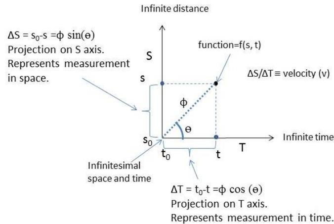
Figure 6 The space-time diagram similar to Figure 1 that represents a flash of light that happened at a position  $s_0$  in space and  $t_0$  in time. Notice that the axes are switched as compared to Figure 1 to correspond with the definition of velocity,  $v \stackrel{\text{def}}{=} \Delta S / \Delta T$ . Notice also that rather than considering the origin to be zero, it is considered to be infinitesimal. There is no meaning assigned to negative space or negative time.
