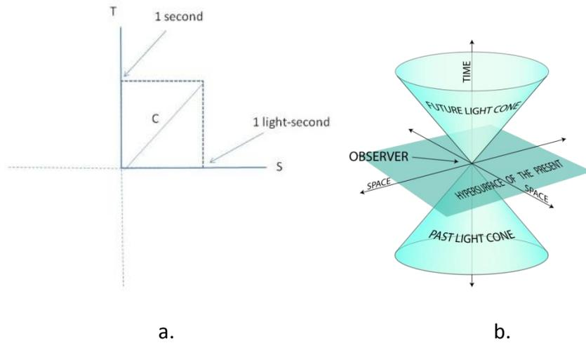
Figure 1 (a) A normalized plot of time vs. space that illustrates the point that light travels one unit of distance (light-second) in one unit of time (second) (b) Minkowski's interpretation of the time vs. space plot, expanded to include the past as negative time and the future as positive time. This is an abstract representation since space is shown as two dimensions, an anomaly that was dodged by calling it the event horizon, an "hyperspace" of the present.
