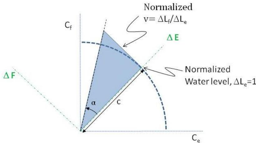
Figure 15 The variable level is superimposed (conformally map) on the same graph (scale) as fullness and emptiness. The angle is referenced to zero change in fullness and the magnitude is referenced to the conversion factor,  $c$ . A non-zero angle represents motion of the level (filling or emptying). The magnitude of  $v$  is zero when the fill rate is zero.
