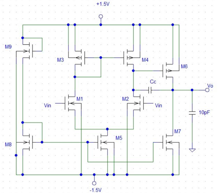
Figure 3. Selected microelectronic op-amp topology based on [6].
