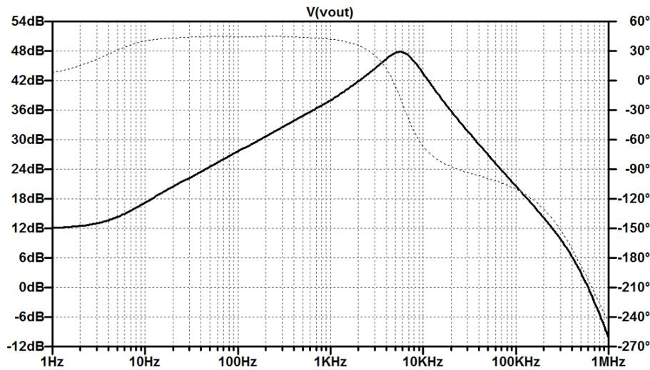
Figure 2. Magnitude (solid line) and phase (dashed line) spectra of a fractional-order differentiator of order  $\alpha = 0.5$ .
