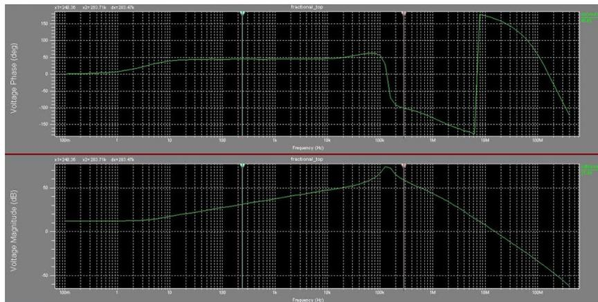
Figure 6. Frequency response of the designed analog CMOS semi-differentiator.
