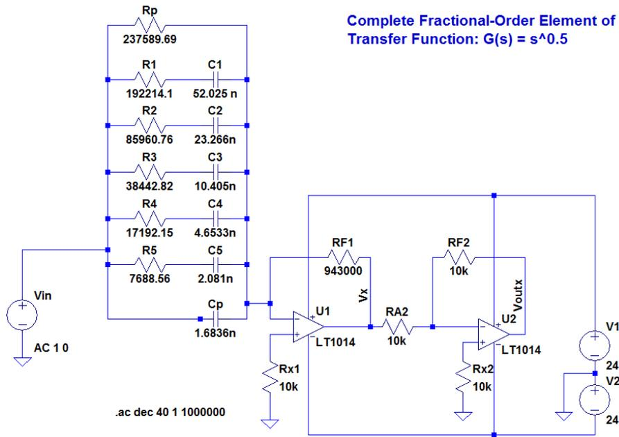
Figure 1. Analog circuit design of a fractional-order differentiator of order  $\alpha = 0.5$ .
