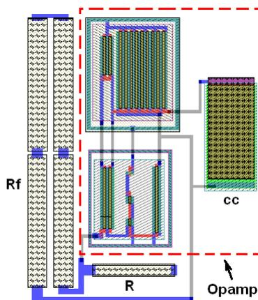
Figure 4. Example layout of an inverting op-amp with a gain of 20.
