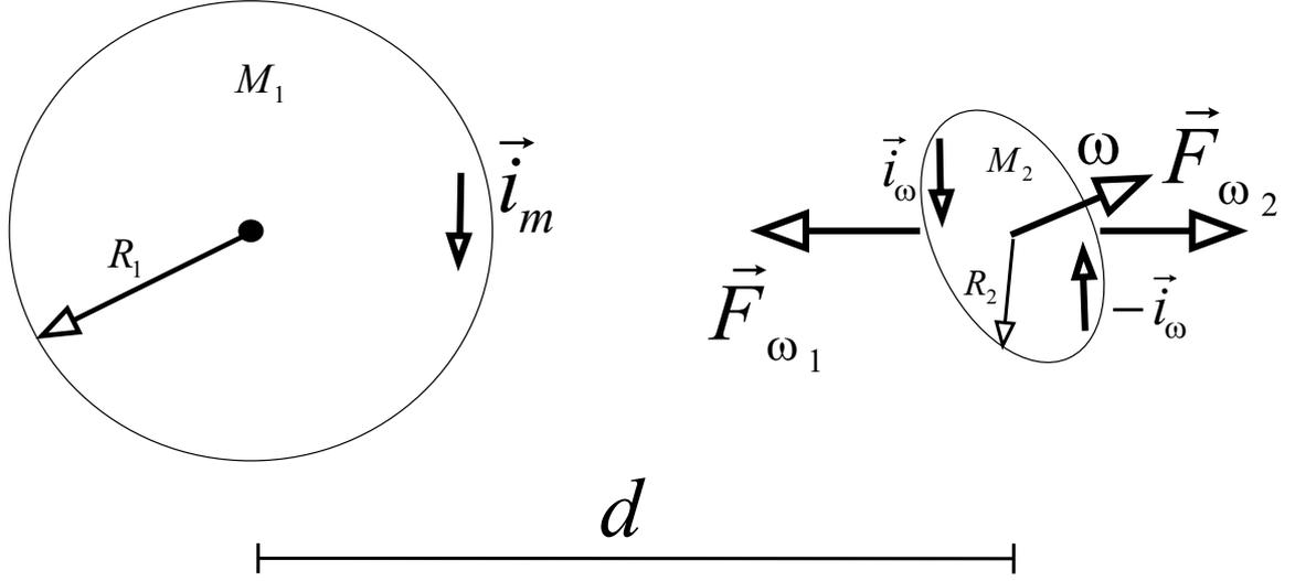
Figure 17: Gyroscopic precession.
