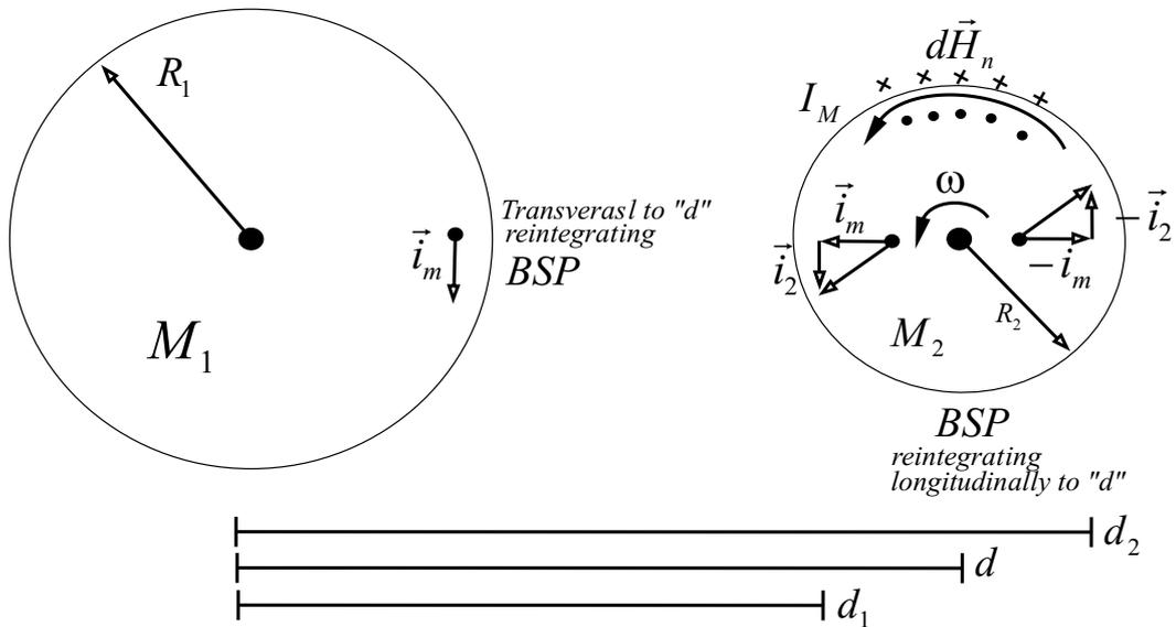
Figure 9: Induced current  $I_M$  and field  $dH_n$  on a rotating neutral body.
