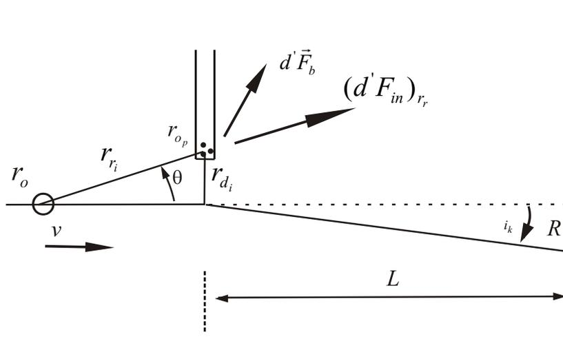
Figure 11: Force induced on a BSP at a bending edge by a BSP moving with speed  $v$ .
