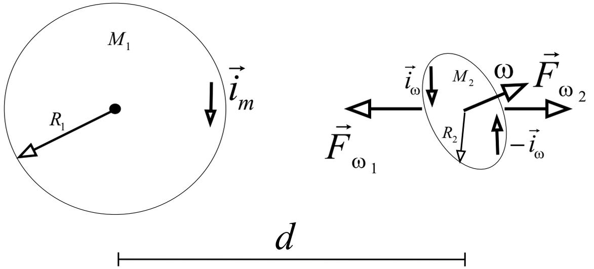
Figure 10: Gyroscopic precession.
