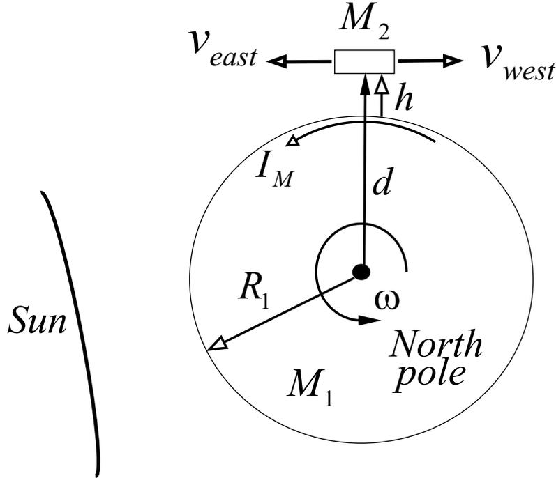
Figure 14: Influence of gravitation on clocks frequency.
