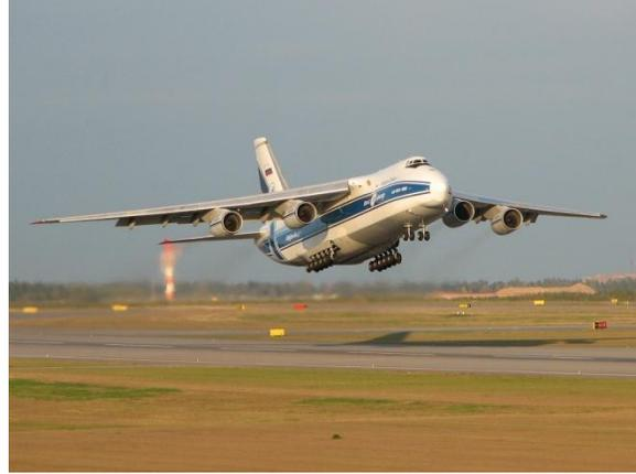
Aircraft AN-124. Weight is 402 tons, payload is 150 tons.
