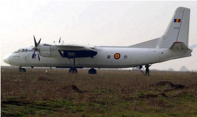
Aircraft AN-24. Weight is 21 tons, passengers 48, produced 1362 pieces.
