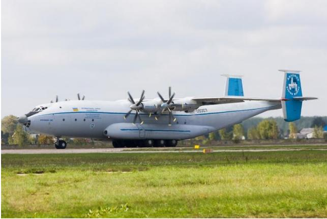
Aircraft AN-22. Weight is 205 tons, payload is 60 tons. Produced 56 pieces.
