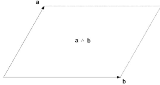
Fig. 1 Two vectors  $\vec{a}$  and  $\vec{b}$  define the bivector  $\vec{a} \wedge \vec{b}$ .
