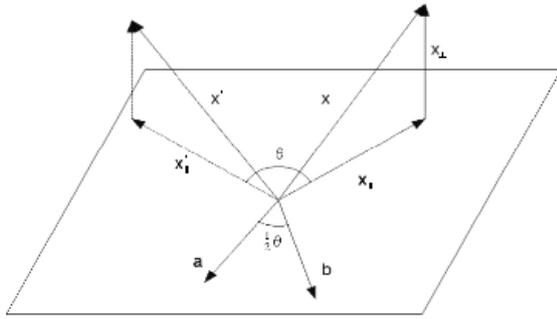
Fig. 3 Rotation of vector  $\vec{x}$  through the angle  $\theta$  around an axis perpendicular to vectors  $\vec{a}$  and  $\vec{b}$ . Note that the rotation is through twice the angle  $\theta/2$  between vectors  $\vec{a}$  and  $\vec{b}$ .
