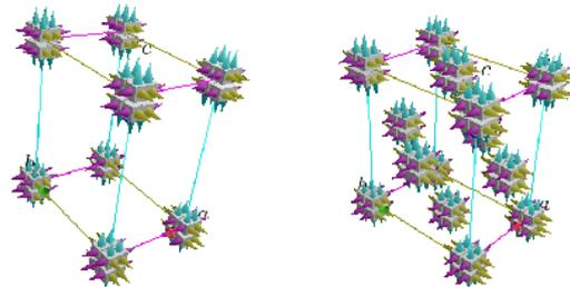
Fig. 8 Unit crystal cells related to orthorhombic point group No. 8 (22), of the space groups No. 47 ( $P22$ ) and No. 69 ( $F22$ ), as displayed with the Space Group Visualizer [7].
