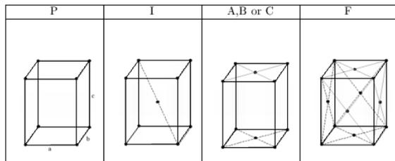
Fig.5 Orthorhombic Bravais lattices, with  $|\vec{a}| \neq |\vec{b}| \neq |\vec{c}| \neq |\vec{a}|$ , and with  $\vec{a} \perp \vec{b} \perp \vec{c} \perp \vec{a}$ .
