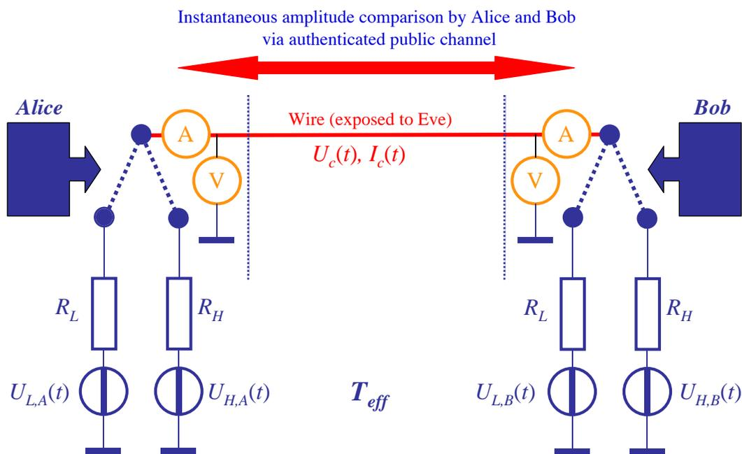
**Figure 3. KLJN system minimally armed against invasive (active) attacks, including the man-in-the-middle-attack.** Alice and Bob measure the instantaneous channel voltage and current amplitudes and compare them via an authenticated public channel. In this way, they learn all the information Eve can have. Additions to prevent hacking—such as line filters, blinding detectors, *etc*—are not shown. The notation is the same as in Fig. 1.
