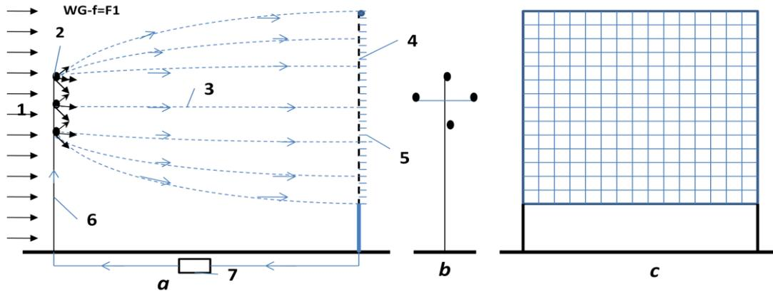
**Fig.1.** One version of Electron Wind Electric Generator (EABG). *a* – side view of the installation; *b* – front view of the electron injector column; *c* – front view of the collect net. *Notations:* 1 is wind; 2 is electron injector; 3 is trajectories of electrons; 4 is net collecting the electrons; 5 is conductive leaves (metallic foil, for example, aluminum foil); 6 is column (post) for supporting of the electron injectors; 7 is the outer electric load.
