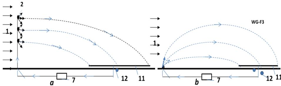
**Fig.3.** The horizontal conductivity film as collector of electrons. *a* – injectors in column; *b* - injectors at Earth surface. *Notations:* 11 - conductivity film (for example, aluminum foil); 12 (optional) positive isolated charge (for example, electrets).
