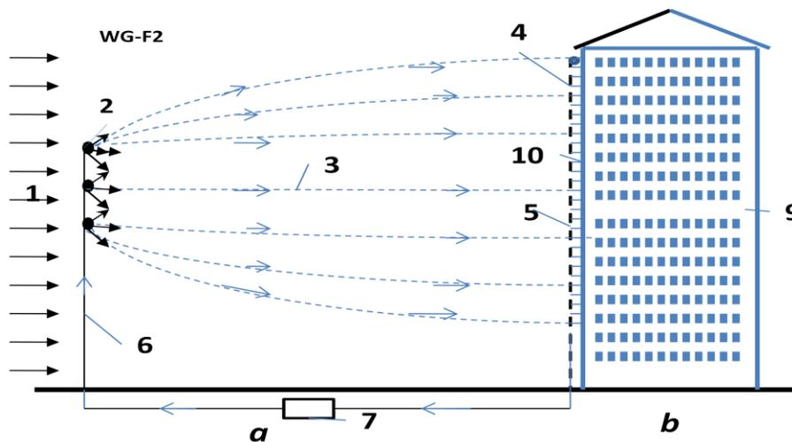
**Fig.2.** Using the building walls as the collector (net) for electrons.
