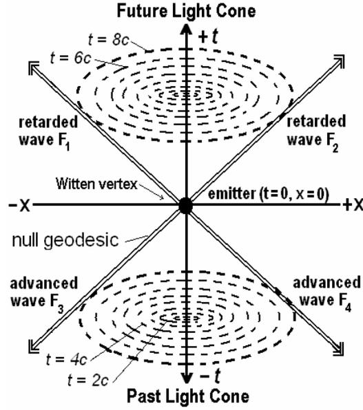
**Figure 6** 4D Minkowski light-cone of advanced and retarded waves (Eq. 1) emitted from a locus at  $(x,t) = (0,0)$ . Adapted from concepts of Cramer [21].
