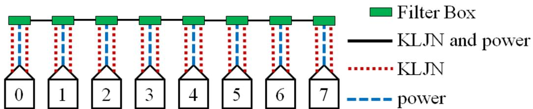
**Figure 5.** Example for network of size  $N=7$ . Each host is connected to a filter box and the filters boxes are connected to the power grid. Note how each host has three wire connections to its filter box.
