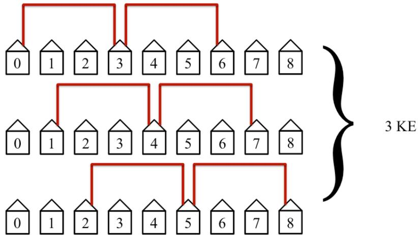
**Figure17.** The third step in the protocol connects the third nearest neighbors. This step requires 3 KEs to complete.
