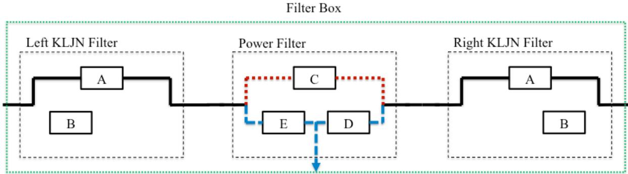
**Figure 6.** The filter box of the inactive host (when it is not executing KLJN key exchange): State 1. Everything is passing between left and right and the host can access only the power. Filter A is passing everything (shorted). Filter B is disconnected. Filter C is passing  $B_{kljn}$  only. Filters E and D are passing  $f_p$  only.
