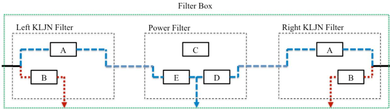
**Figure 7.** The filter box of the active host (when it is executing a KLJN key exchange): *State 2*. The power is passing between left and right but the KLJN band is not and the left and right KLJN units are separated while doing a key exchange toward left and right.
