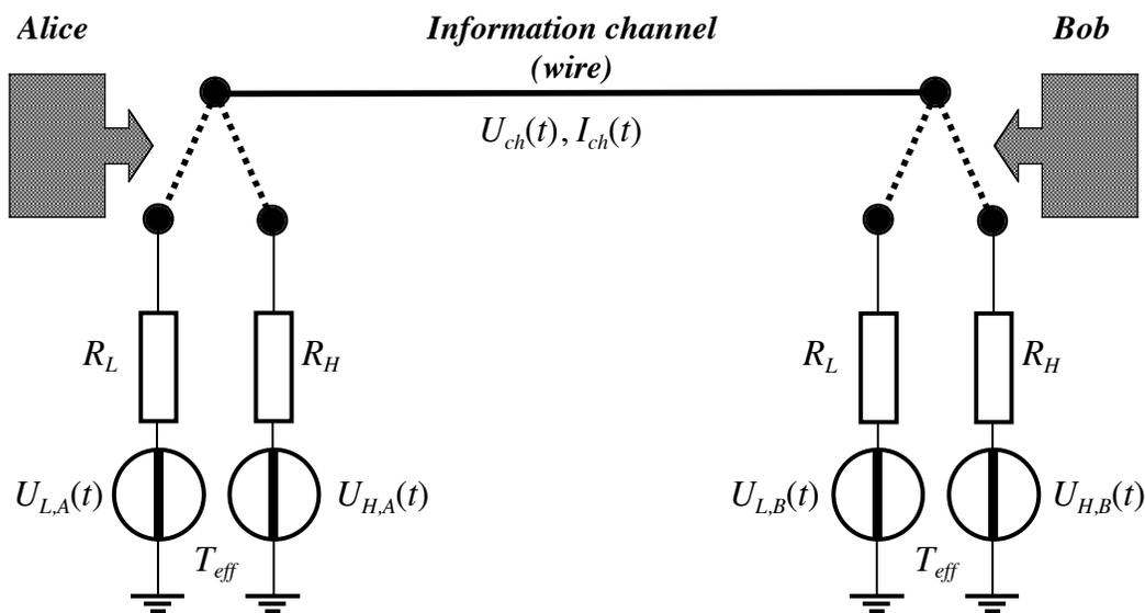
**Figure 1.** The core of the idealized KLJN key scheme [22-25]. This simple system is secure only against passive attacks in the idealized case (mathematical limit). Security enhancements (including filters) to provide protection against invasive attacks [22-25] and against other types of vulnerabilities are not shown. In practical applications electronic noise generators emulate an enhanced Johnson noise with a publicly agreed high effective temperature.
