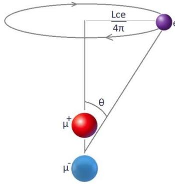
In this “Cone” model of an electron, the orbital angular momentum  $L$  equals to spin  $s = \frac{h}{4\pi}$ , and the orbital magnetic dipole momentum equals to  $\frac{\mu_B}{2}$ . The dipole momentum of the magnetic dipole also equals to  $\frac{\mu_B}{2}$  (3.2.13). The total magnetic momentum then equals to  $\mu_B$  – the Bohr magneton.
