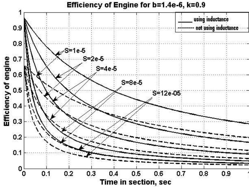
**Fig.5.** Comparison of efficiency the RailGan (dash line) and HABE (full line) via outer current time  $\tau$  for different Ohm resistance  $S = \rho/2s$ .
