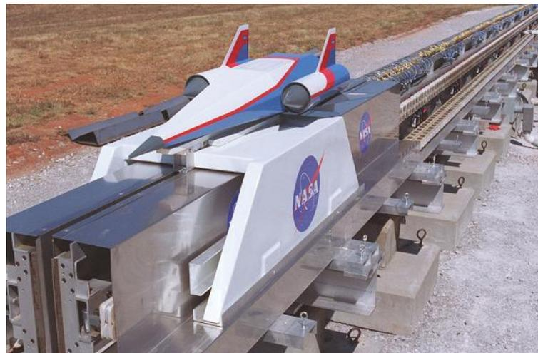
**Fig.2.** Catapult for aircraft. Credit NASA.
