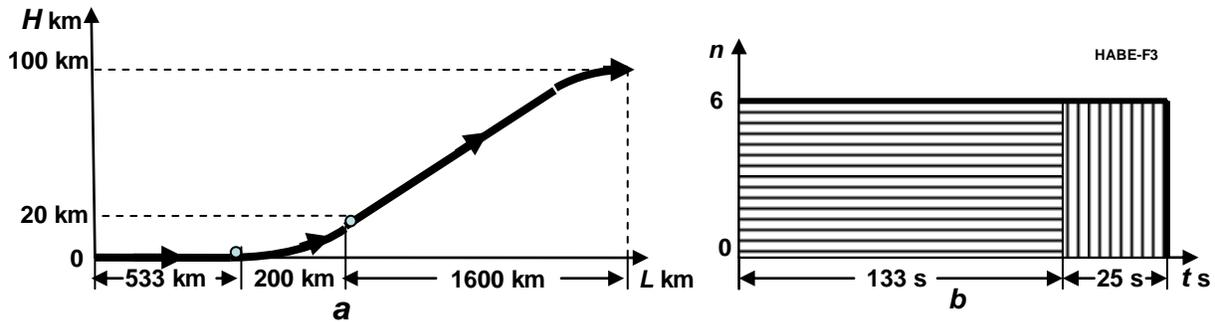
**Fig.7.** Launch trajectory of space ship (a) and diagram of overload (b).
