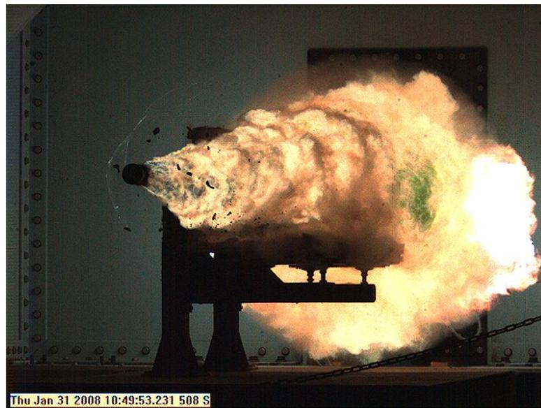
**Fig. 1.** Railgun. Credit NAVY. Naval Surface Warfare Center test firing in January 2008, leaving a plume of plasma behind the projectile. The Gun has a small shell and gigantic plasma flash. The 70 - 80% of energy lost in this flash overheats the rails and does not allow immediately making the next shot.
