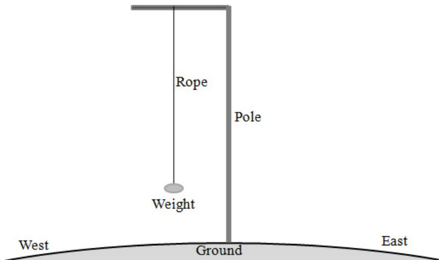
**Figure 12: Experimental frame on measuring the oscillation of weight.** The longer the rope, the more easily observable the oscillation of the weight.
