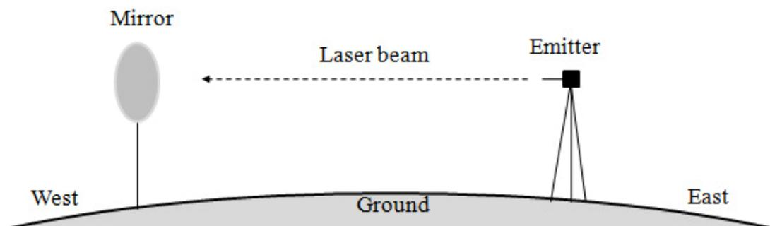
**Figure 13: Experimental frame on measuring the oscillation of laser beam.** The more distant between the two sites, the more easily observable the oscillation of the laser beam in the mirror.
