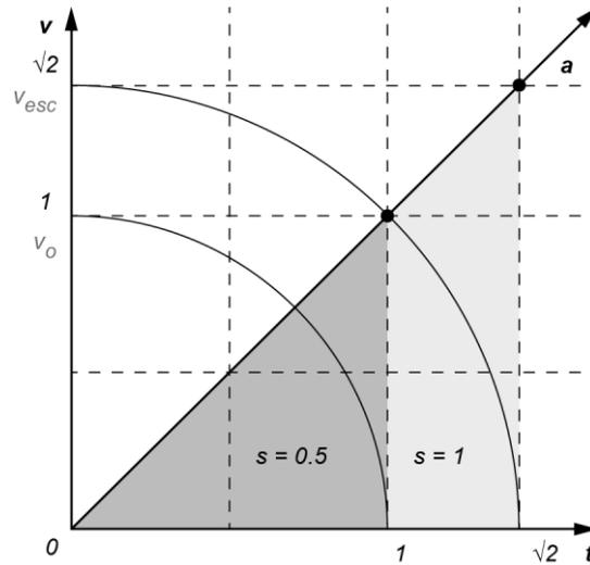
**Figure 1.1.2.c** Graphic representation of the velocity of the body in a free fall measured on the whole and half of the distance travelled. Their difference is a factor of  $\sqrt{2}$ , which is equivalent to the relation between orbital and escape velocities.
