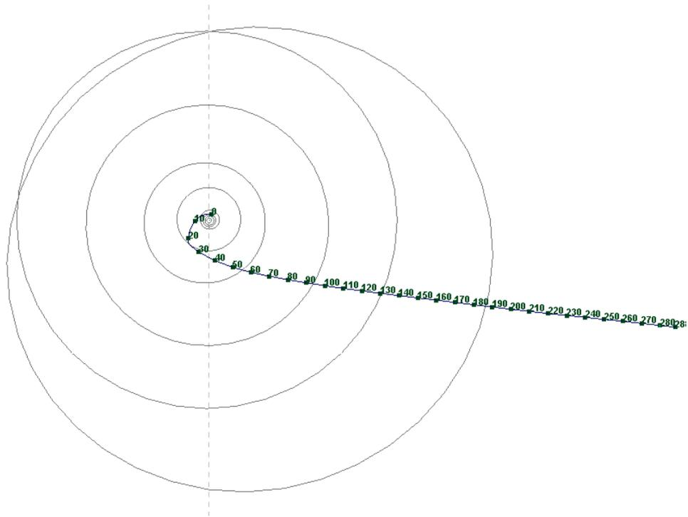
**Figure 1.2.3.5** Trajectory of the probe divided into regions of annual distance travelled
