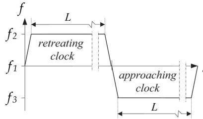
FIGURE 3. Frequency changes of clock  $A$
