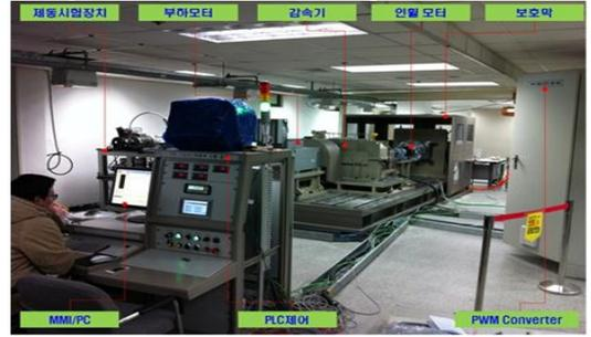
Fig. 7. Control algorithm test using HIL simulator
