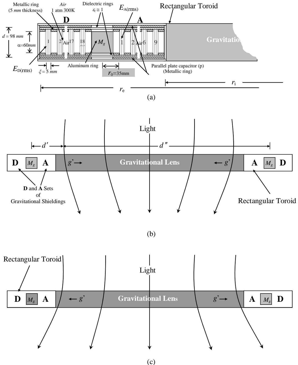
Fig. 3 – Artificial Gravitational Lens. (a) Cross-section of the Artificial Gravitational Lens. (b) Cross-section of a *Convergent* Gravitational Lens. The light rays are *gravitationally repelled* from the inner edge of toroid (c) Cross-section of a *Divergent* Gravitational Lens. The light rays are *gravitationally attracted* to the inner edge of toroid.
