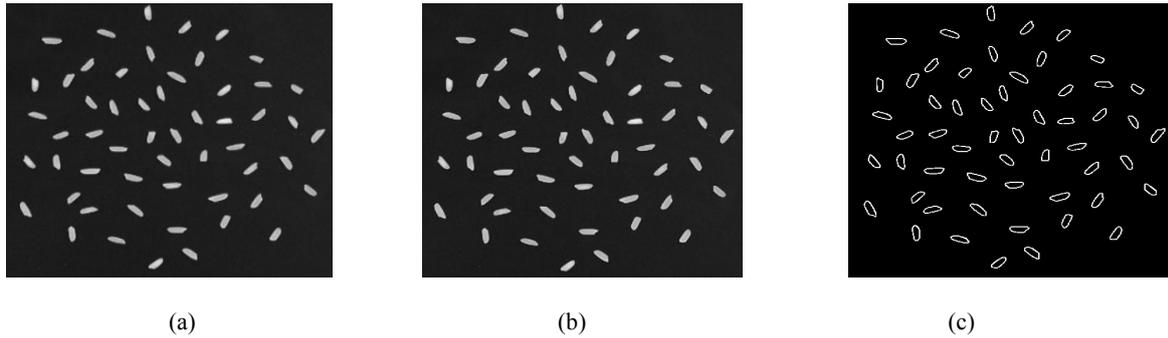
Figure 6 (a) RGB (b) Gray-scale (c) Edge detected image of one of the sample of Gujarat-17 Rice seed.
