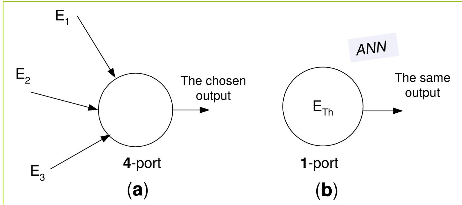
'(a)' is a *linear* 4-port if we accept (recognize) all of the ports. If we recognize only one port, i.e. start to see this whole circuit as a 1-port, then the circuit becomes *ANN*, in the sense of (1).
