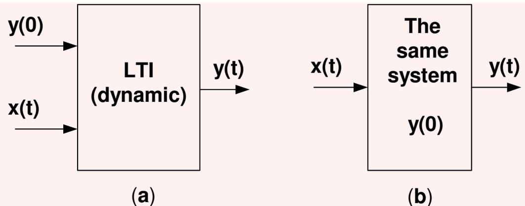
Notice that in the domain of the Laplace variable, the interpretation of the initial values of state variables as “inputs” is even a standard one.
