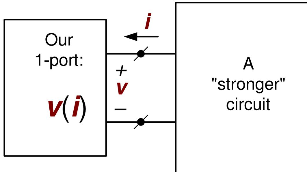
A 1-port is used for creation of a nonlinear resistor
