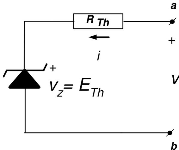
This is the partial (not for any  $\text{sign}[i]$ ), **passive mode** equivalence that is important for creation of nonlinear resistors  $v(i)$ , see Slide 11.
