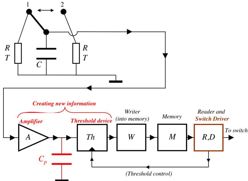
Figure 7. Possible realization of an electrical Maxwell demon. Some of the elements can be joined in other realizations, but the energy dissipation sources described here remain.
