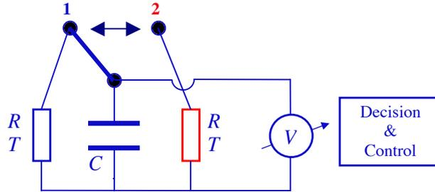
Figure 1. Electrical Maxwell demon with Johnson noise in stage 1. The temperature  $T$  is the same in both resistors. The thick line indicates the moving part of the switch and the double-ended arrow the switching positions.
