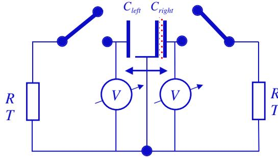
Figure 10. Arbitrarily chosen starting point of the cycle for the electrical Szilard engine. The piston is at the right end and the capacitor at the right has the work charge  $Q_w$ . The corresponding electrical energy is  $E_w \gg kT/2$ .
