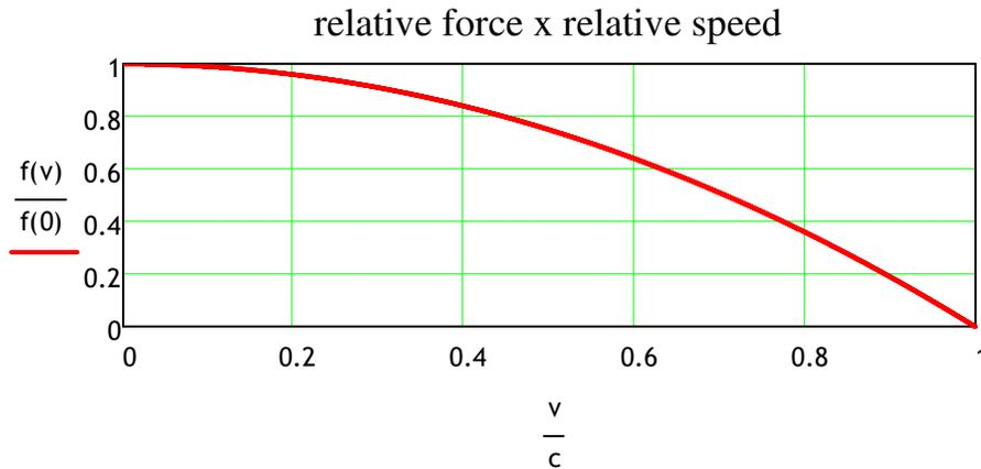
$$a = \frac{c^2 - v^2}{2 \cdot m} \quad (10) \quad \Leftarrow \text{maximum possible acceleration at speed } v$$
