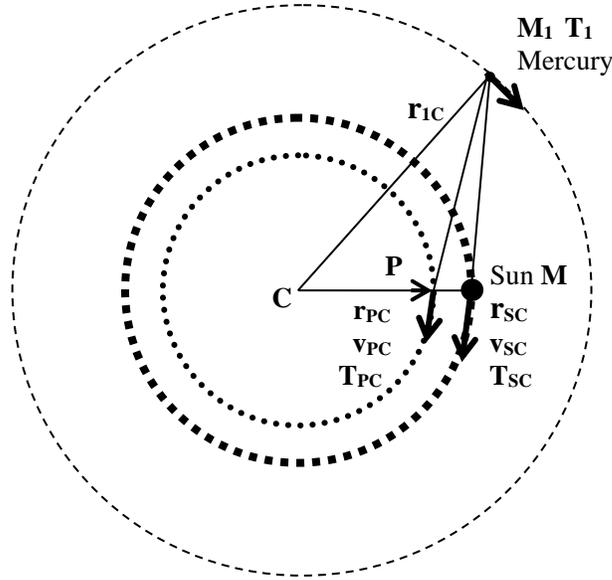
**Fig. 2** Schematic diagram showing the Sun moving slowly around the barycentre at C. Mercury is considered to be orbiting the effective centre of gravity at P, between C and the Sun.
