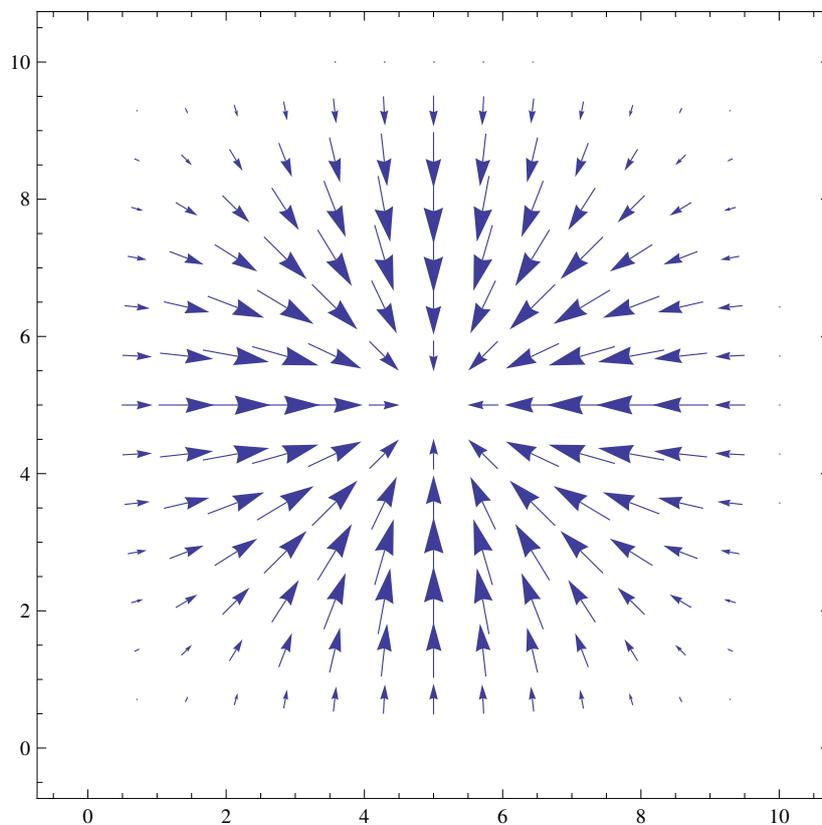
Figure 7: Direction of the particles' acceleration when in contact with the oscillating surface as the plate's acceleration approaches infinity. Simulation parameters:  $1 \times 1$  mode produced on a  $10(\text{m}) \times 10(\text{m})$  plate.
