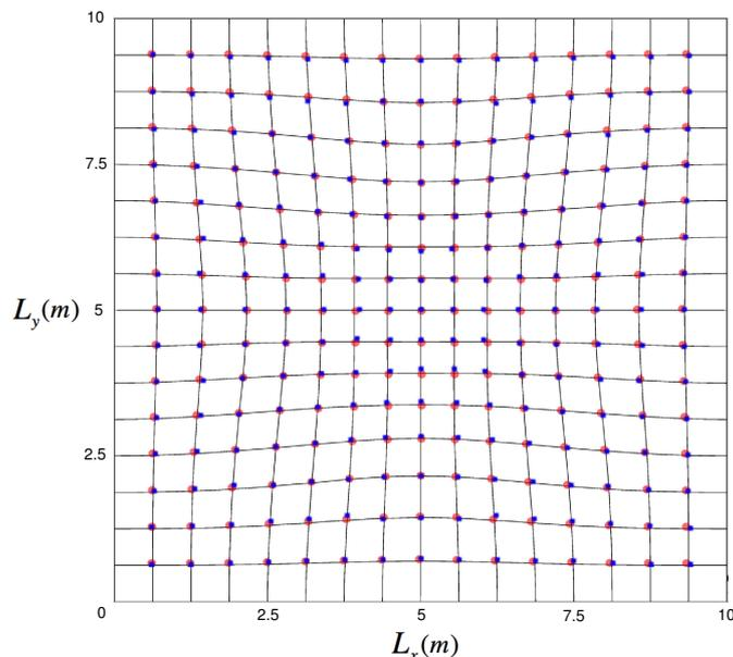
Figure 4: Particle displacement for  $\mu_i = 0.1$ . The red dots at the points of intersection in the  $17 \times 17$  grid show the positions of particles predicted using Eq. 7 after 8 s. The blue dots show the positions of particles obtained from the numerical simulation.
