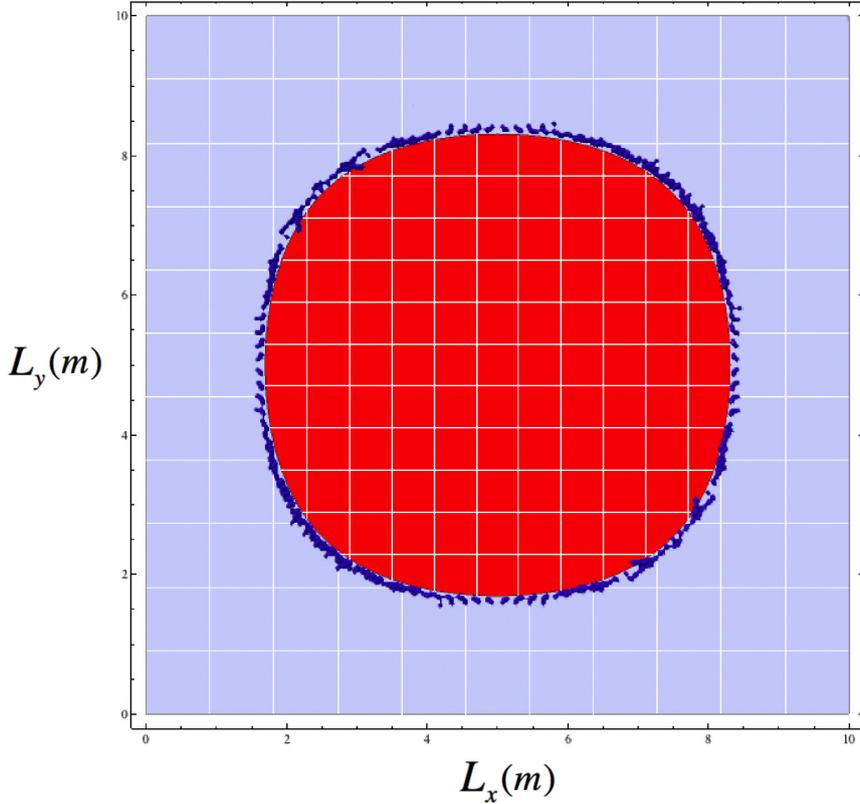
Figure 5: Particle ejection area (red). The blue dots surrounding the red area show the particle positions obtained from the numerical simulation. Stationary particles in the light blue region were ignored in the figure.
