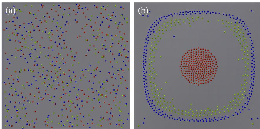
Figure 9: Numerical simulation of a sorting mechanism based on the particle-damping coefficient  $c$ . The particles had the following values of  $c$ : 0.1 (blue), 0.5 (green), and 0.9 (red). (a) Initial random positions of the particles. (b) Positions of the particles after 150 s
