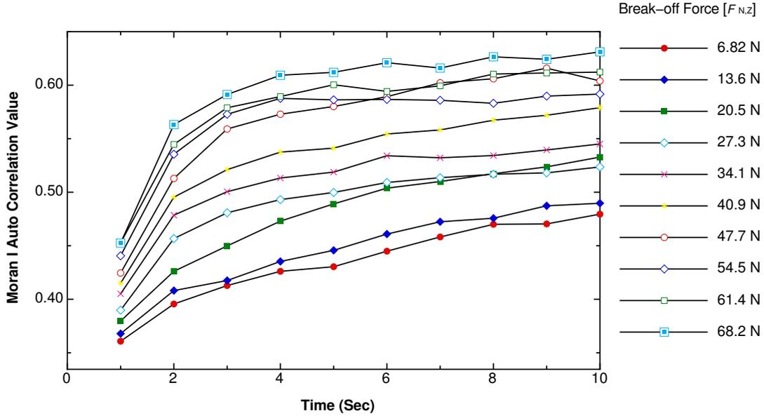
Figure 1: Effect of *adhesion* on the rate of pattern formation: Moran's I values of patterns formed from 1 to 10 s for various values of the break-off force (simulation parameters:  $\mu_i = 0.1$ ,  $f = 9$  Hz, and 10,000 particles).
