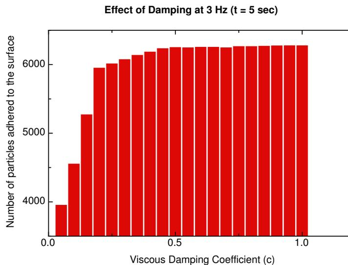
Figure 8: Effect of damping on the number of particles adhered to the surface. Both temporarily attached and permanently attached particles (due to adhesion and damping) were included in the count. The simulation was initiated with 10,000 particles. Other particles from the y-axis count either bounced (they were temporarily ejected) or were completely ejected from plate. Simulation parameters:  $F_{N,Z} = 6.82\text{N}$ , and  $\mu_i = 0.1$ .
