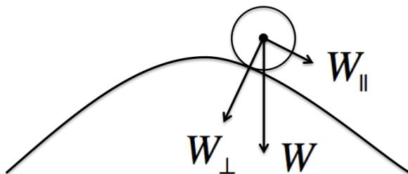
Figure 3: Weight  $W$  of a particle and its components ( $W_{\parallel}$  and  $W_{\perp}$ ) when it is in contact with a surface.
