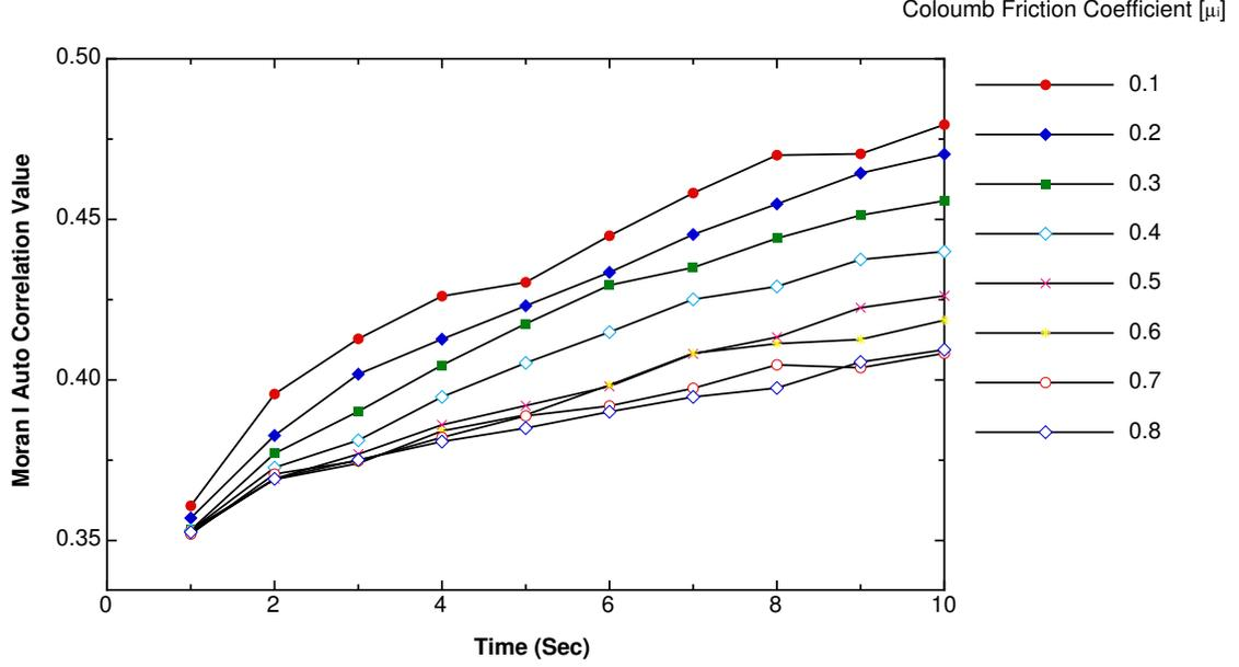
Figure 2: Effect of *friction* on the rate of pattern formation: Moran’s I values of patterns formed from 1 to 10 s for various values of the Coulomb friction coefficient (simulation parameters:  $F_{N,Z} = 6.82\text{N}$ ,  $f = 9\text{ Hz}$  and 10,000 particles).
