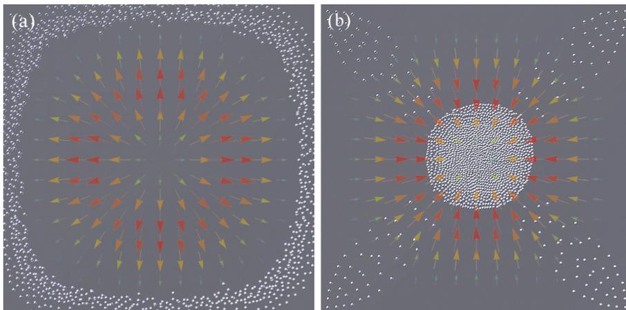
Figure 6: Using adhesion to alternate between standard and inverse Chladni patterns. The position of particles is shown at  $t = 100$  s. (a)  $F_{N,Z} = 1\text{N}$  standard pattern of collection at the nodes. (b)  $F_{N,Z} = 50\text{N}$  inverse pattern of collection at the antinodes. Simulation parameters:  $1 \times 1$  mode, 10,000 particles,  $\omega_{kl} = \frac{\sqrt{2}}{2}$  and  $\Gamma m = F_{N,Z\text{critical}} = 19.74\text{N}$ .
