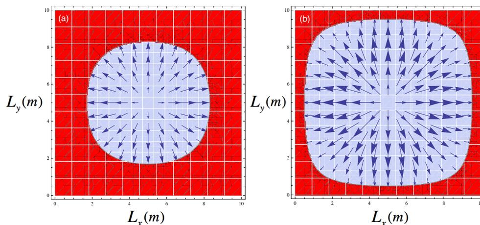
Figure 10: The effect of particle damping on the force (blue vectors) exerted on a bouncing particle within the ejection area (light blue). a) Forces experienced by particles with high damping coefficients. (b) Forces experienced by particles with low damping coefficients. These vector plots are just illustrations, and the difference between the ejection areas has been exaggerated; this figure is used only for qualitative analysis.
