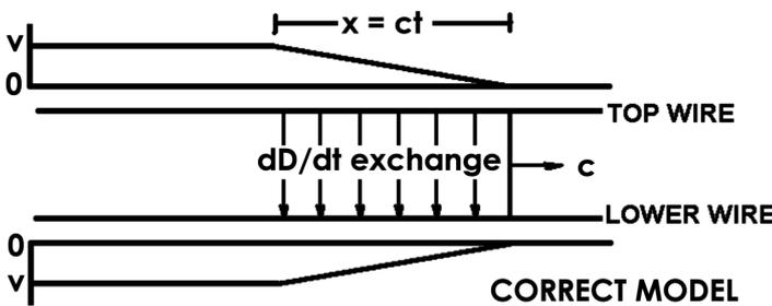
Mechanism for electric current flow: accelerating electrons radiate radio to opposite wire (exchange) Each signal is inversion of the other: "cancellation".
