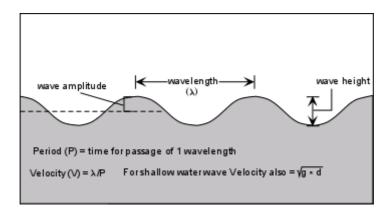
At the stage of free propagation of the wave in the open ocean at large depth, tsunami is known to be of  $\sim 1$  meter height [3]. When the wave enters shallow water, it slows down and its amplitude (height) increases, *see* [2]:
