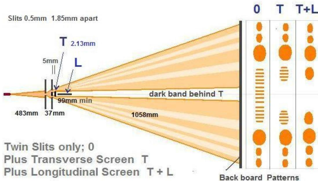
Overlapping light paths blocked by transvers screen T. 5mm behind twin slits (with edges in dark bands) Part of interference pattern remains. When lateral screen L is introduced in the dark band behind T the remaining interference patten is lost.
