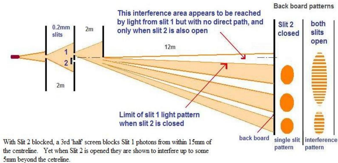
**Figure 10b. Double Slit Variation b.** A third screen edge is positioned on the centreline. Interference still occurs in the central area inaccessible to photons from slit 1 without an exceptional refraction angle. This is however consistent with new oscillators or waves propagated at the edge of the third screen by HFP and WFS. (Fleagle 'Separated Pattern').
