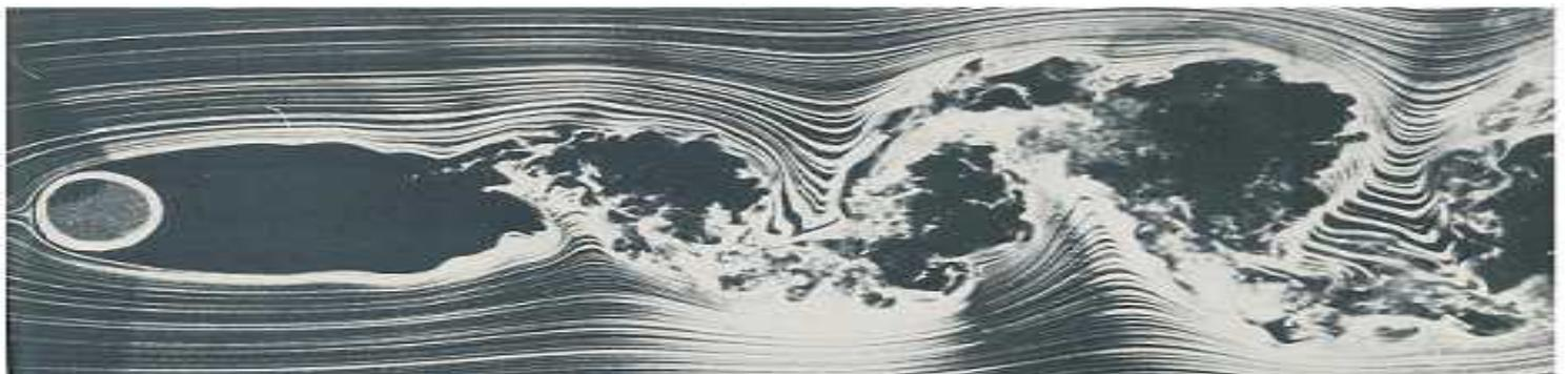
(a) Visualizing turbulent cylinder wake at  $Re = 10000$
