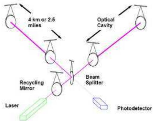
**Fig. 5 Schematic diagram of Laser Interferometer Gravitational-wave Observatory**
