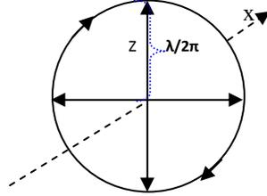
*The figure represents transverse view of a propagating electromagnetic wave. The vertical and the horizontal lines stand for two perpendicular oscillations having phase difference of  $\frac{\lambda}{2\pi}$ . Here the circular velocity is taken as  $c$ .*
