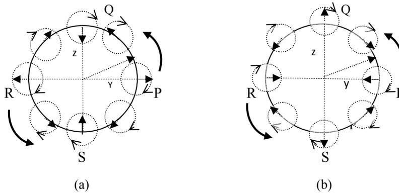
(a) shows the case where the rotation of the helical wave is in the anti-clockwise direction while the electric field rotates in the opposite direction. The field has positive component  $\xi_y$  at P on the y-axis and becomes  $-\xi_z$  at Q, then  $-\xi_y$  at R and  $\xi_z$  at S. (b) represents the case with the same direction of rotation but with the phase of of the electric vector differing from that of case (a) by  $\pi$ .
