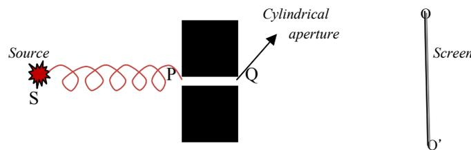
*S is a very weak monochromatic microwave source. PQ is the cylindrical adjustable aperture while OO' represents the screen which measures the intensity of the microwave falling on it. If the helical wave hypothesis is correct, the aperture could block all waves having wave length more than  $2\pi r$ .*
