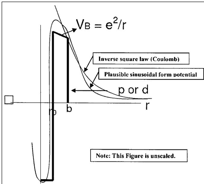
Figure 1. Potential for Coulomb barrier reversal for STTBA, reprinted with permission from Takahashi.<sup>2</sup>
