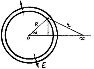
Figure 7: Two-dimensional capacitor
